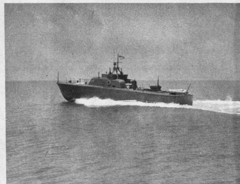
Most modern and effective of U. S. air-sea rescue craft is the 85-ft. picket boat. Trim and powerful in appearance, it relies on a high speed of 35 knots to bring air-crew casualties ashore as quickly as possible.
